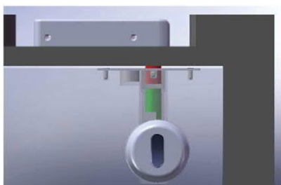
Deadbolt which is unable to release the bolt during power failure.
