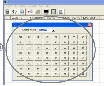
Instructions: Appendix - " Elevator Open Door " function is able to set open the door or test individual floors to make sure each relay is work normally.
