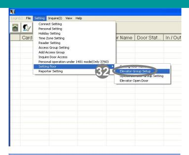
Instructions: Elevator Groups Setup, this helps to define a certain person as a elevator group, which is to set the rules for a certain person allows to get in/out for an indicate floor, on the other hand if not joined floor cards are not allow to enter door.
