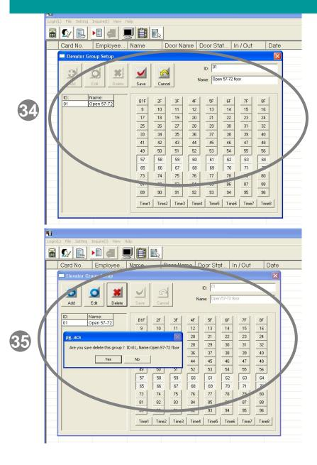
Instructions: Elevator Groups Setup, this helps to define a certain person as a elevator group, which is to set the rules for a certain person allows to get in/out for an indicate floor, on the other hand if not joined floor cards are not allow to enter door.
