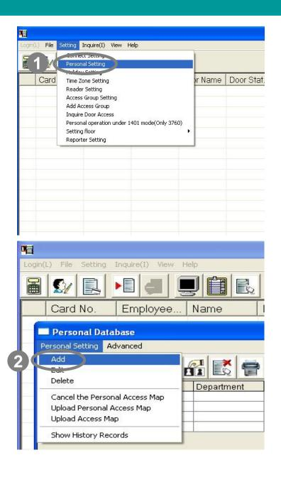
The example illustrates: The ELE series access software not only support access control function but also joined the lift access control, following below steps for the operation setting details
