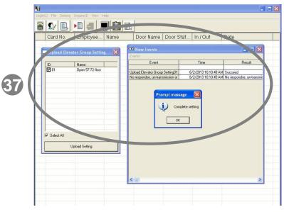
37 :Select the upper-left corner of the floor box group, click the bottom-left of the "Upload Setting" and pop out "View Events" window, make sure that the "Upload Elevator Group" result are "Succeed ",finally, click" OK "button to the end.
