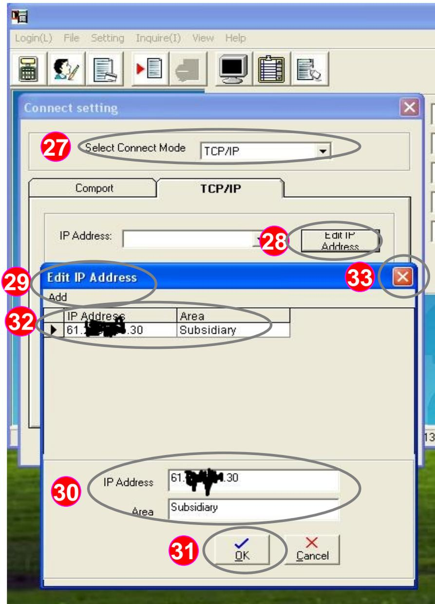
**Instruction: Login to parent company access control software and do the subsidiary of the PC-T100 + PP-6750V card reader connection settings**
