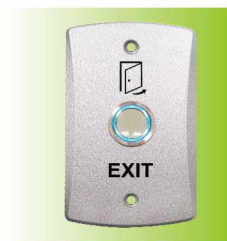
PBT-09 115(L) x 70(W) x 5(H)mm With Blue LED N.O. / N.C. / COM.
